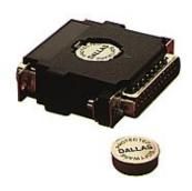
*NOTE:* Before the FastCAM® programs can be run you "MUST" attach your FastLOC DONGLE to your Printer PORT. If a printer is connected to your PC, attach it to the "LPT1 *Printer Port"* where the printer is connected now. You then attach your Printer Cable to the FastLOC DONGLE.
