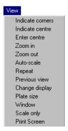
The VIEW MENU allows the manipulation of the view on the graphics screen. By using the view menu the programmer can zoom in for a close up view of a section of the part, change the scale of the part, or look at a previous view. The view menu appears both in FastCAM and FastPLOT. In FastPLOT the view menu also has nesting functions.
