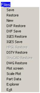
The Files MENU contains menu items for Saving and Restoring FastCAM geometry files. These files are automatically assigned the file extension of (.CAM). Contained in this menu are also the menu items for the importation of CAD (DXF) and (IGES) files.
