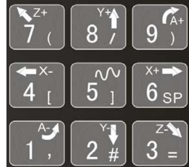
In manual mode, 5# key can be used to switch the manual speed and rapid traverse speed. The rapid traverse speed of every axis depends on comprehensive parameter 009-012 (rapid traverse speed setting). After switching to rapid traverse speed, the manual speed of the position interface will be highlighted, while the actual speed of the position interface is sampled from the moving speed of current axis. This value can truly reflect the moving speed of current axis (unit: mm/min);
