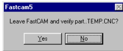
16. FastCAM will close and FastPLOT will open displaying the generated NC code. The program can now be saved to a floppy disk or sent to the cutting machine using a DNC link if available.
